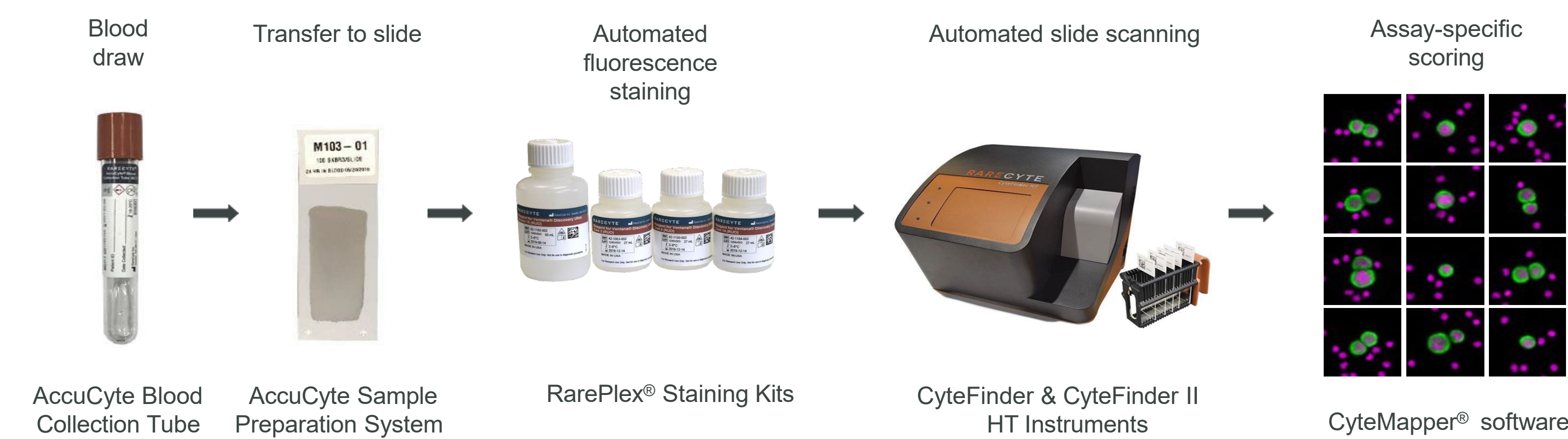
Figure 1. RareCyte platform workflow. Blood is collected into AccuCyte Blood Collection Tubes (BCTs). Nucleated blood cells are processed to slides using the AccuCyte Sample Preparation System. Slides are stained with assay-specific RareCyte staining kits. Slides are scanned using the CyteFinder Instrument and images are analyzed using CyteMapper software and analysis tools. Cells are analyzed by a trained reviewer, and cell biomarker status is determined with a fluorescence intensity threshold.
