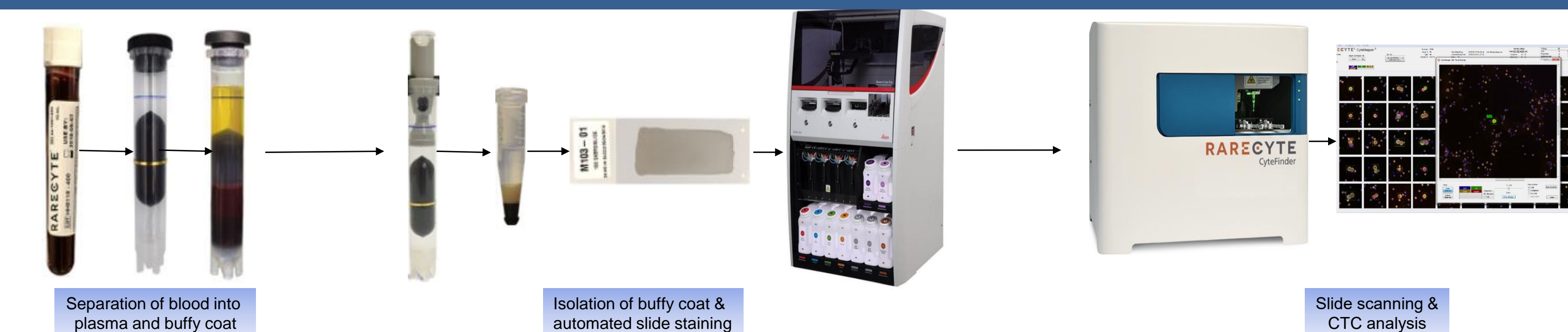
Workflow for quantification of CTCs from blood samples. Each blood collection tube with 7.5ml of blood is transferred to the AccuCyte® blood separation tube and centrifuged at 3000g for 25 min. Plasma is separated and displacement fluid is added along with the buffy coat isolation tube and centrifuged at 1000g for 20 min. Transfer fluid is used to resuspend the isolated buffy coat and 8 slides are made for every blood collection tube. These slides are then stained using the CTC biomarker staining kits using a Leica® automated stainer. Stained slides are banked at -20°C or scanned using the CyteFinder® system and CTC are quantified using the CyteFinder® software. (Image source: www.rarecye.com and www.leicabiosystems.com )
